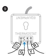
Insert the wires you just disconnected into the C Wire Adapter terminals.
