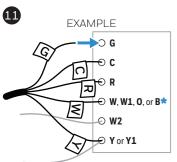
Connect the wires from the "Equipment" labelled side of the C Wire Adapter to the matching terminals on the control board.
