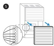
Open HVAC system's cover to reveal the control board.
