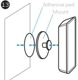
Before mounting, check to make sure surface is clean enough to ensure good adhesion.
