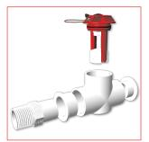
FIG. C: ON DRAIN PAN Insert the threaded fitting (5) into the drain pan. Glue the threaded fitting (5) into the 1"  $\times$  3/4" reducer bushing (3) and the pipe tee (2). Glue the PVC cap (4) into the pipe tee (2). Insert the sensor assembly (1) into the pipe tee (2) and press firmly. Do not glue the sensor assembly on to the pipe. Ensure that the sensor is not tilted more than 30°. (Refer to FIG. D)
