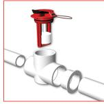
FIG. A: PIPE INLINE Glue the 1" x ¾" reducer bushing (3) to the pipe tee (2). Glue pipes to the ¾" ports. Insert the sensor assembly (1) into the pipe tee and press firmly. Do not glue sensor assembly on to the pipe. Ensure that the sensor is not tilted more than 30°. (Refer to FIG. D)
