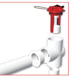
FIG. B: 90 DEGREE Glue the 1" x ¾" reducer bushing (3) to the pipe tee (2). Glue pipes to the ¾" ports. Insert the sensor assembly (1) into the pipe tee (2) and press firmly. Do not glue the sensor assembly on to the pipe. Ensure that the sensor is not tilted more than 30°. (Refer to FIG. D)
