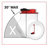
FIG. D: SENSOR TILT THRESHOLD
