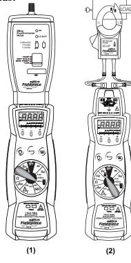
Connect to Fieldpiece accessory heads by simply attaching them to the top of meter (1) or attach remotely through leads (2). For most heads, move dial to range shown (1). For the AAC clamp (ACH4), move dial to VAC range (2). Accessory heads not evaluated in UL61010-1 certification.
