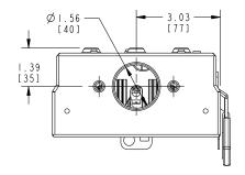
TYPE I ENCLOSURES: COLD ROLLED STEEL .045" THICK FINISH: ANSI GREY #61 PAINT
