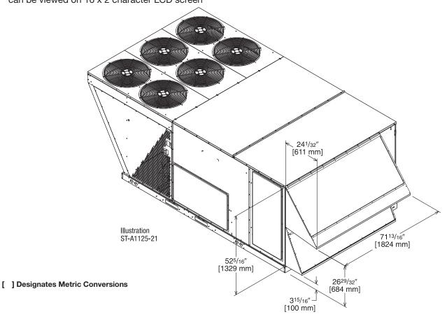
**ECONOMIZER FOR HORIZONTAL DUCT INSTALLATION**Field Installed Only
