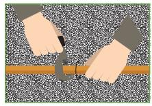
**STEP 1 - CUT COPPER TUBE** Cut copper tube using a commercially available tube cutter. Verify tube cutter is properly maintained and wheel is sharp. **DO NOT** use any type of saw as this creates a sharp surface that will cut the o-ring.
