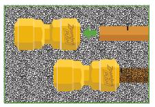
**STEP 6 - PUSH INTO FITTING** Push the tube into the fitting. Use the mark to assure insertion depth and secure fit.
