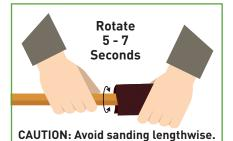
STEP 3 - SAND and CLEAN ALL tubing must be SANDED and CLEANED. Use a general purpose hand pad or sand cloth. SAND tube in RADIAL DIRECTION as shown with arrows for 5 - 7 seconds or 10 - 14 times backand-forth. Remove residual debris from tube end.
