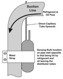
As recommended in Section 7B-I, the TXV sensing bulb should be mounted in a horizontal plane in relation to the suction/vapor line. However, some installation configurations may require that the sensing bulb be mounted vertically. In this instance, place the bulb opposite the piping wall being hit by refrigerant and oil leaving the distributor tubes, and with capillary tubes directed upwards as shown in Fig. 7B-3.
