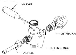
Fig 7B-1. Components of a typical TXV assembly
