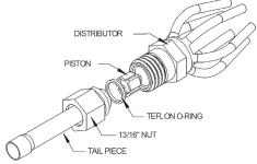
Fig 7A-1. Flowrator assembly components
