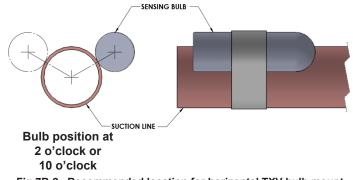
The TXV sensing bulb SHOULD be mounted on the suction line approximately 6" from the TXV or coil housing using the metal clamp provided. In order to obtain a good temperature reading and correct superheat control, the TXV sensing bulb must conform to ALL of the following criteria:
