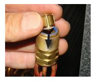
6. Replace the piston with one of the correct size. Do not force the new piston into the body. Make sure the piston moves freely in body.
