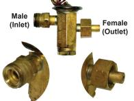
**III-4.** Remove the valve from the box and note the location of the inlet side (threaded male port) and the outlet side (female swivel nut port).
