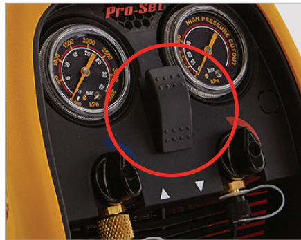
Ignition proof power switch
