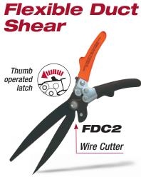
The Flex Duct Shear (FDC2) Cuts insulated flexible round duct and also cuts the duct liner's wire rib coil. Pointed bottom blade easily pierces duct to start cut. Heavy duty wire cutter is located away from scissor blades. Thumb operated latch ensures that sharpened blade edges stay closed when not in use.
